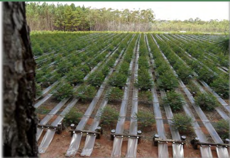
37% throughfall exclusion using plastic sheets
