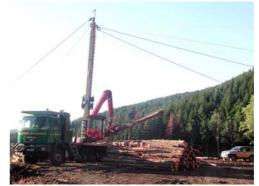
The cable cranes are now replacing the long distanced skyline equipment.
