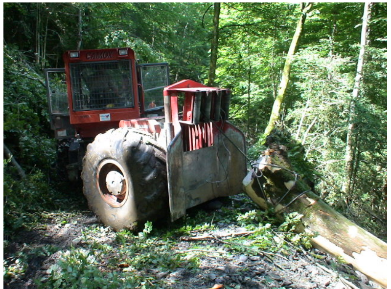
Figure 1 Synthetic rope is a strong innovation for log skidding in mountainous areas
