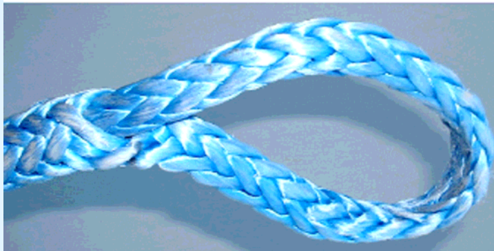
Figure 7: Eyed splice (an end connection)
