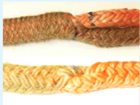
Figure 8: Long splice (fixing of 2 divided pieces)
